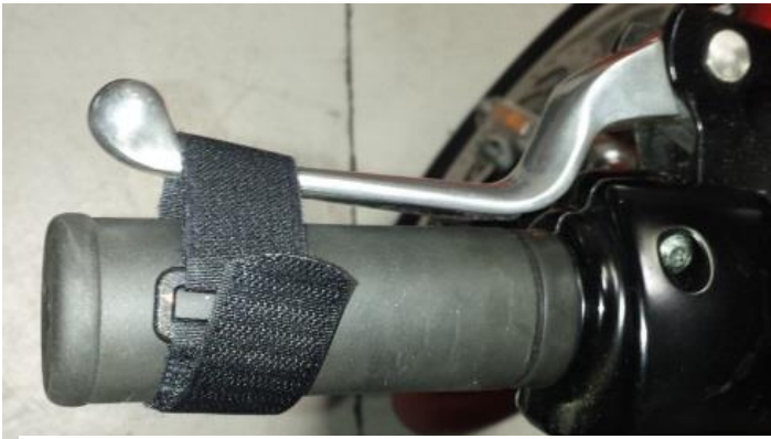
Clutch Lever Strap: to prevent unwanted launching.
