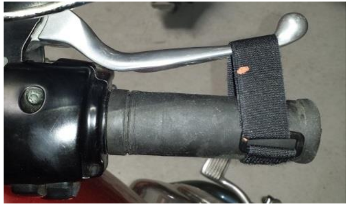
Brake Lever Strap: for use as a parking brake.
