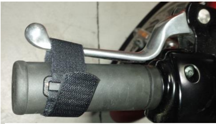
Clutch Lever Strap: to prevent unwanted launching.
