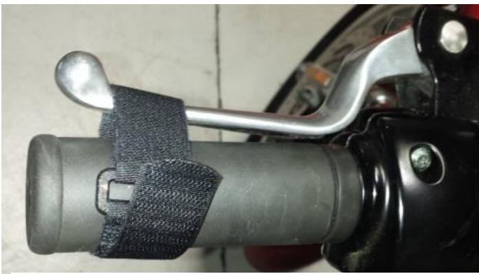
Clutch Lever Strap: to prevent unwanted launching.
