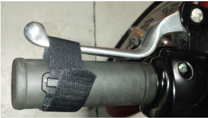
Clutch Lever Strap: to prevent unwanted launching.
