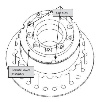
**20.** Using a pair of mechanics gloves (the edges of the ring can be sharp and may cut you), install the retaining ring into the Rekluse Center Clutch ring groove.
