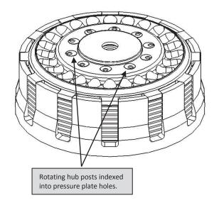
30. While holding down the pressure plate so it is indexed with the basket and 10 rotating hub posts properly, place the Rekluse top plate over the Rekluse pressure plate and thread in 2 torx head screws180° across from one another. Lightly tighten the 2 screws to secure the Rekluse top plate.
