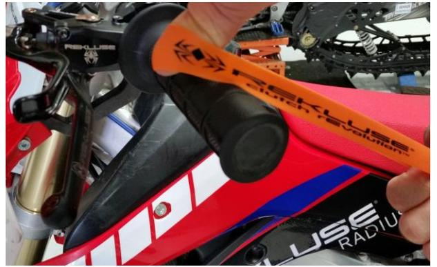
c) While holding the top end of the rubber band against the handlebar, stretch the band downward, then loop it through itself.
