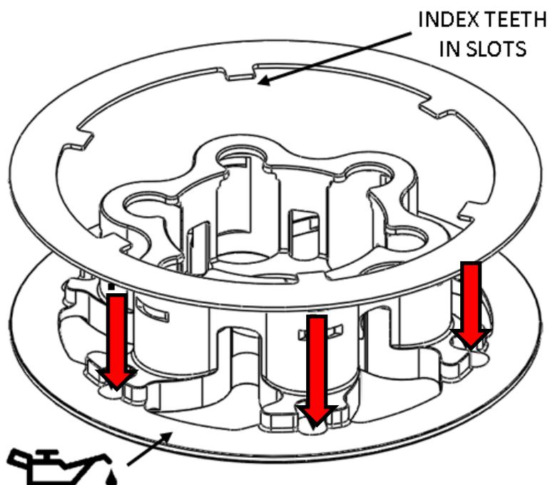
**Note:** Adding a few drops of oil between the pressure plate and lining plate will help them stick together when installing them onto the clutch pack.
