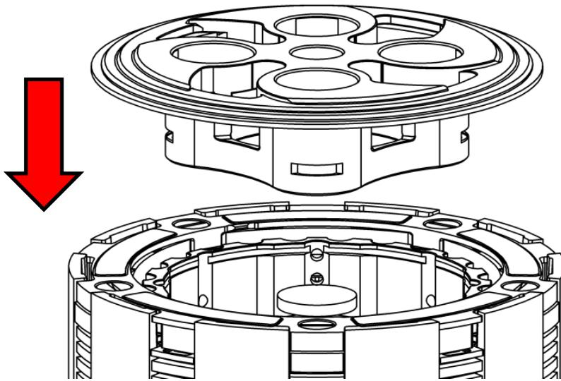
12. Install the Rekluse pressure plate springs, then install the screw sleeves.
