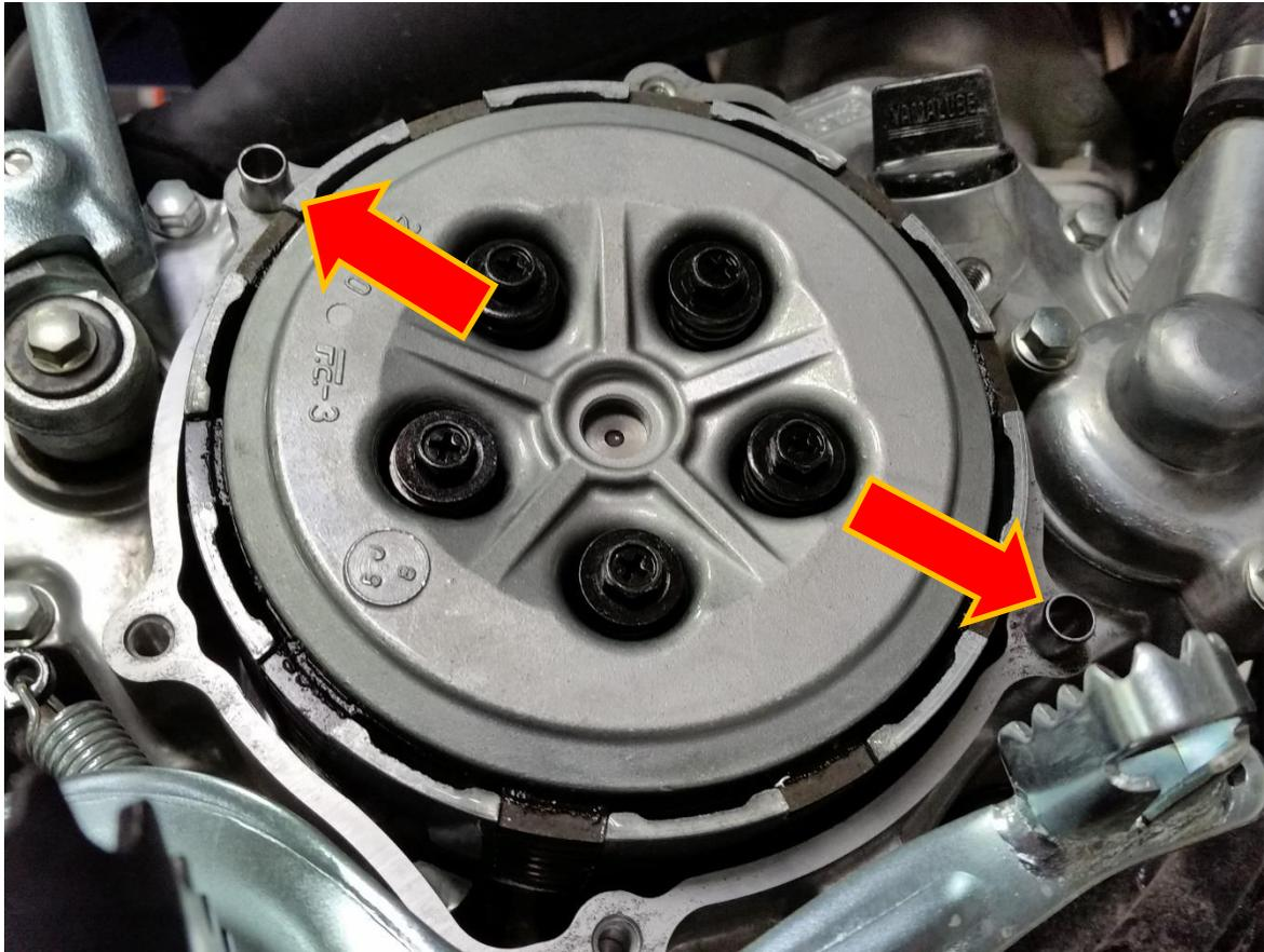
15. Install the OE clutch cover gasket (or install a new gasket) onto the Rekluse clutch cover.
