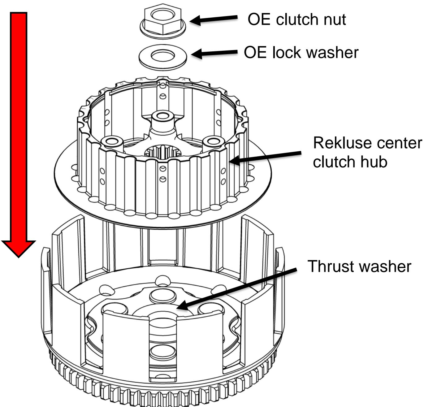
5. Torque the nut to **40 ft-lb (55 N-m)**. **Do not over torque** or the clutch will drag and damage may occur.
