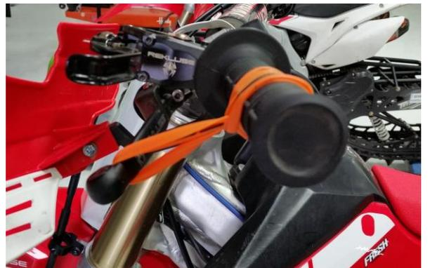
e) While still in **NEUTRAL**, quickly rev the engine between 5,000-7,000 RPM (1/2 to 3/4 throttle), then let it return to idle. The end of the clutch lever **should move in about 1/8" (3mm)** toward the handlebar as you rev the engine. This is your Free Play Gain.
