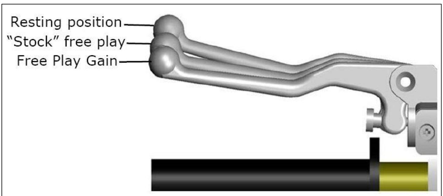
If there is too much Free Play Gain, the installed gap is too small. The bike may drag and stall because it has difficulty disengaging the clutch. It may also be difficult to shift. Too much Free Play Gain will not hurt the clutch, but it will negatively affect clutch performance.
