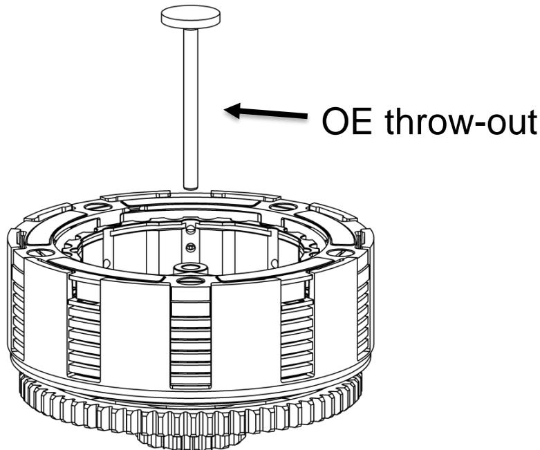
9. On a workbench, turn the Rekluse pressure plate over.
