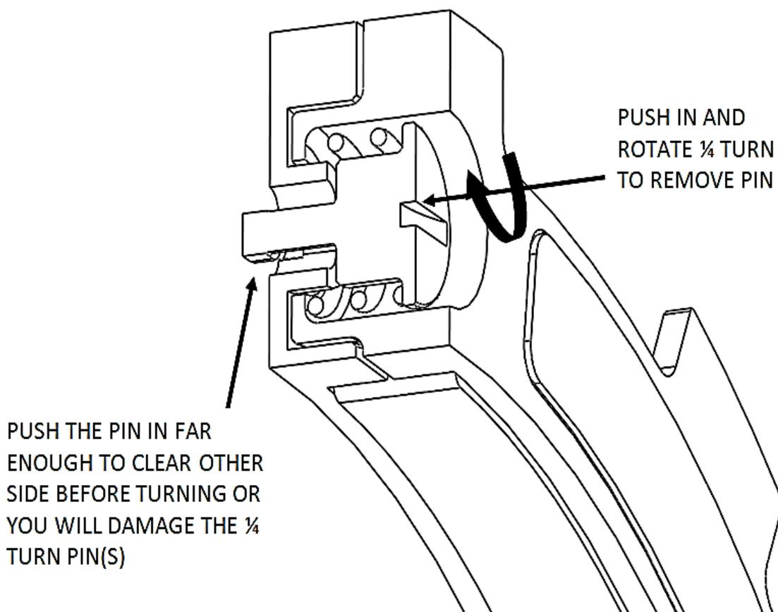
3. Remove the remaining 4 pins and springs of the EXP base.
