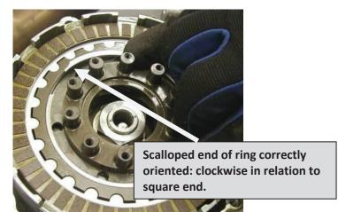
Threading retaining ring into groove
