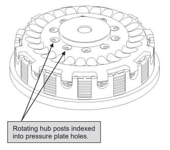
26. While holding down the pressure plate so it is indexed with the basket and 10 rotating hub posts properly, place the Rekluse top plate over the Rekluse pressure plate and thread in 2 of the torx head screws 180° across from one another. Lightly tighten the 2 screws.
