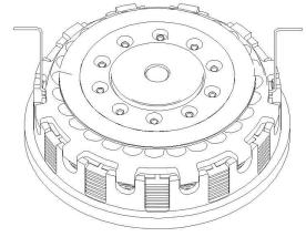
**Note:** A .060" drive plate is included with z-Start Pro Clutch Kit to tighten the Installed Gap. Once the .060" drive plate has been used, and the clutch wears enough so the wire gauges slide in again, the friction disks need to be replaced.
