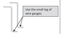
29. If the wire gauges can be slid up and over the pads smoothly, the clutch pack needs adjustment. Swap the thick .060" Rekluse drive plate for the top drive plate. Repeat step 28.
