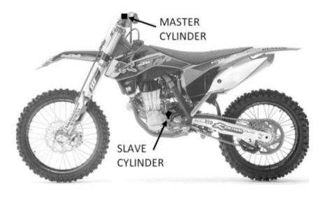
**NOTE:** Some slave cylinders have an 8mm banjo bleeder bolt, a 10mm banjo bleeder bolt, or a straight fluid line. Follow the instructions based on the type of fluid line on your bike.
