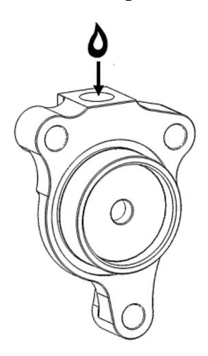
d. Turn the adjuster screw clockwise until it bottoms, keeping the fluid topped off.
