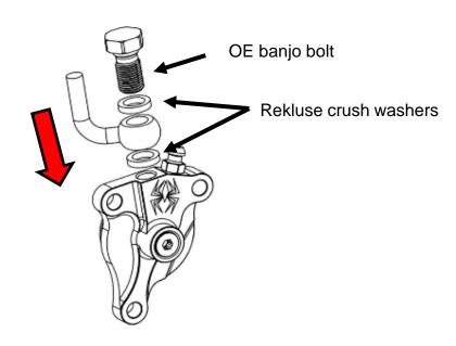
**NOTE:** A quick transfer of the fluid line will result in less bleeding in the following steps.
