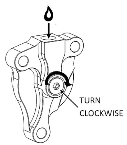
e. Turn the adjuster screw back to the initial position with the top O-ring visible.
