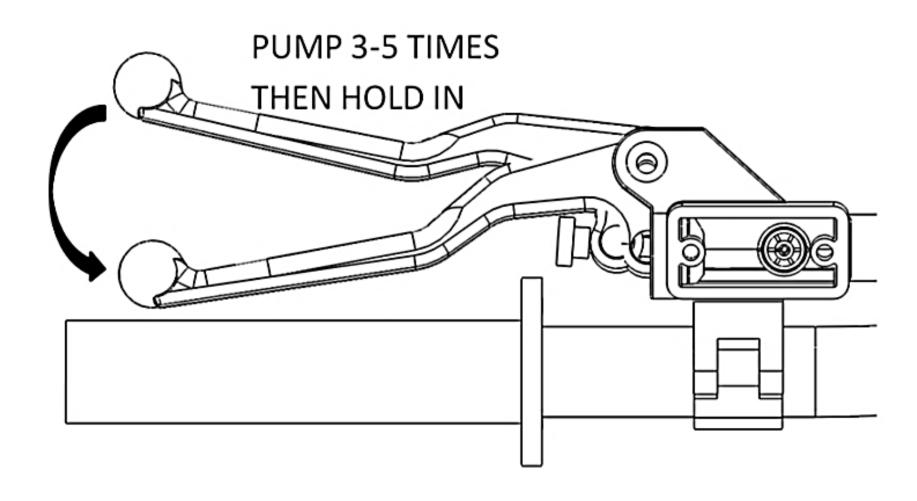
16. Using a 7 mm wrench, open the bleed port. Air and fluid should come out of the bleed tube. Tighten the bleed port.
