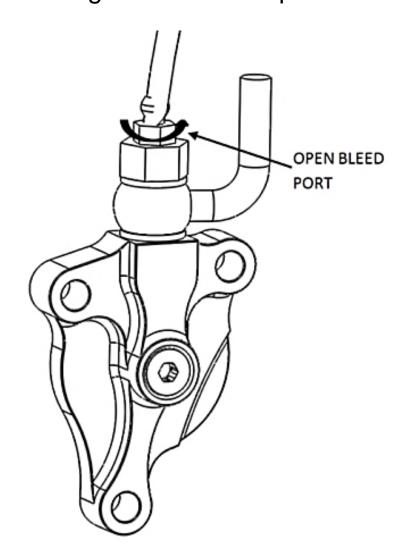
17. Slowly release the clutch lever and check the fluid level in the clutch master cylinder. Add fluid as needed.
