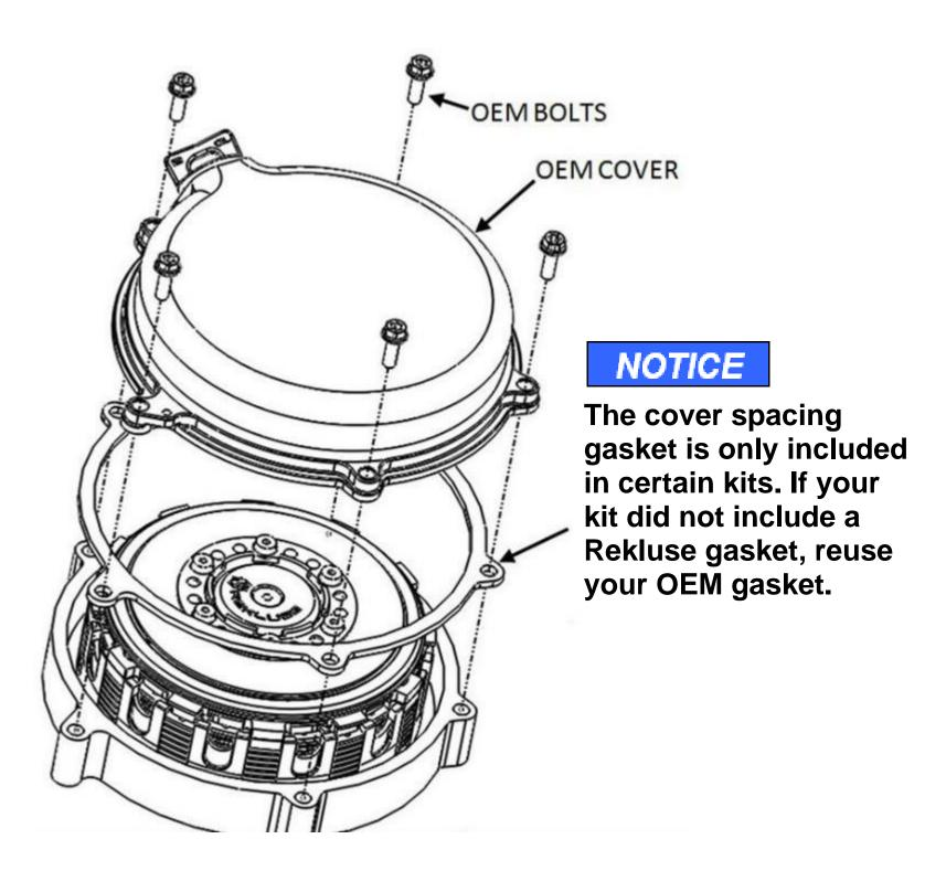
17. Install the clutch cover bolts in their proper OEM location. Lightly tighten the cover bolts in a star pattern. Torque the bolts in small increments before tightening all the bolts. Torque the cover bolts to OEM specification – **7.4** ft-lb (**10** N-m).
