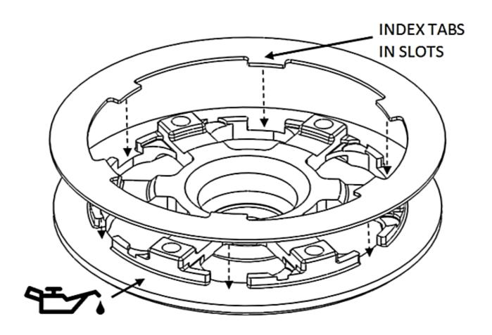
11. Install this pressure plate / lining plate combo, keeping the lining plate against the pressure plate. Hold the pressure plate against the clutch pack until it is bolted down in the later steps
