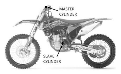
18. On the left side of the bike, while leaving the OE slave cylinder bolted on the engine, use a wrench to remove the banjo bleeder bolt from the OE slave cylinder.
