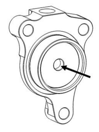
c. Pour clutch fluid into the slave cylinder port.
