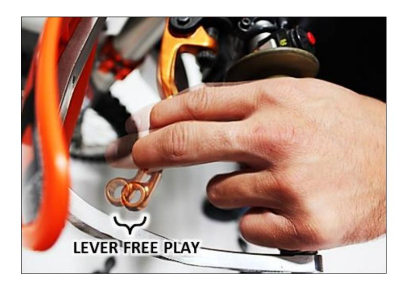
"Free Play Gain" is the increase of lever free play as the auto-clutch engages. This happens when the RPM increase from idle through around 5000 RPM. Free Play Gain is caused by the expansion of the EXP disk which lifts the pressure plate away from the throw-out assembly.
