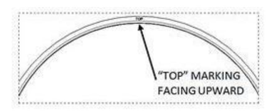
14. Place the OE Belleville spring onto the slider ring, with the rounded dome side facing up.
