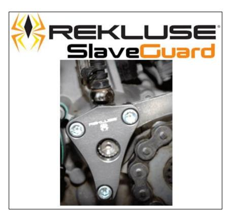
13. Attach the supplied bleed tube to the banjo bolt port and loop it into a suitable catch bottle.
