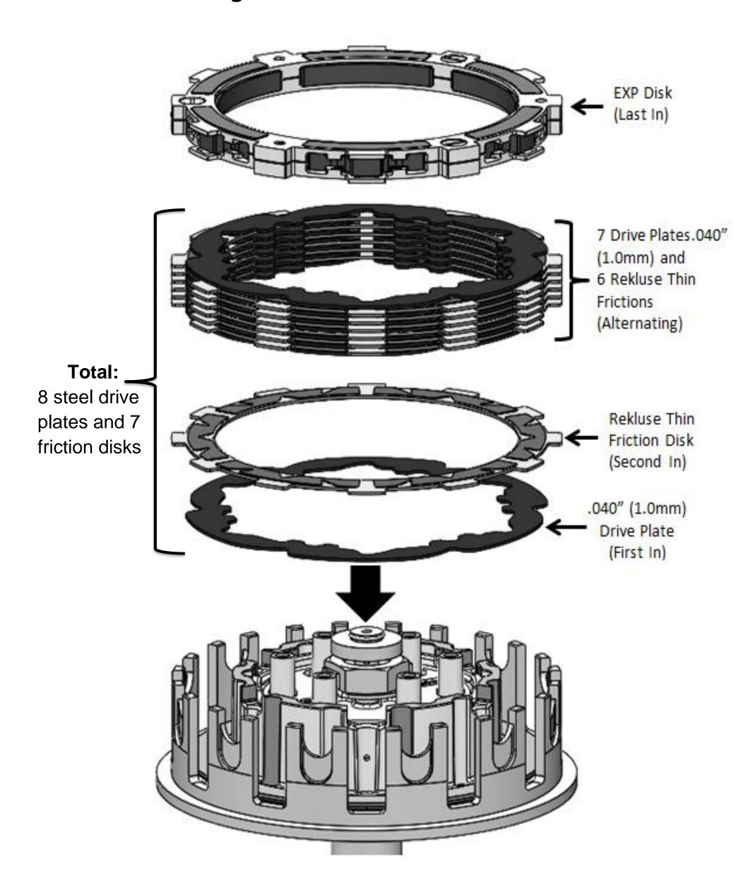
10. Place the Steel Lining Plate onto the Rekluse Pressure Plate. Adding an oil film between them will help them stick together for ease of installation.
