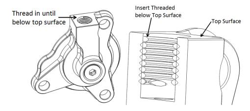
3. Using the needle-nose pliers, bend the thread insert tang up and down until it breaks off and remove it from the adjustable slave cylinder.
