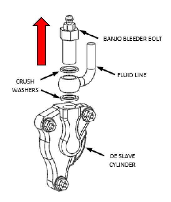
6. Attach the clutch fluid line to the Rekluse slave cylinder using the OE banjo bolt and the 2 new crush washers from Rekluse. Make sure the clutch fluid line is between the 2 crush washers.
