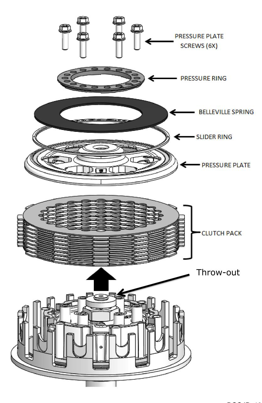
The KTM DDS clutch (a.k.a. Belleville spring clutch) employs a 2-piece damped center hub assembly, as shown. Rekluse clutch products employ the same technology and reuse the OEM rubber dampers.
