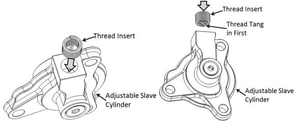
2. Stop when the thread insert is below the top surface of the fluid port. If the insert is not below the surface the crush washers will not seal.
