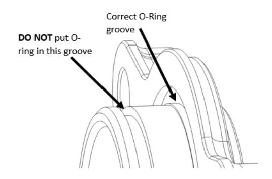
**NOTE:** The Rekluse slave cylinder comes preassembled in the kit. If the parts become separated, assemble them in the following order: Rekluse slave cylinder, O-ring, then the supplied paper gasket.
