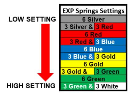
It is **NOT necessary** to disassemble the EXP halves to change springs! To change springs, remove 3 of the ¼-turn pins from one side of the EXP, replace springs, and reinstall ¼-turn pins. Next, flip the EXP disk over and repeat on the other side if necessary. To maintain even pressure when using two different color spring sets, install one color set of 3 on one side of the EXP and the remaining color set of 3 on the other side.
