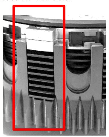
6. Hold a TEC drive plate so that the "shark fin" notches face toward the right. *All the drive plates will follow this orientation.*
