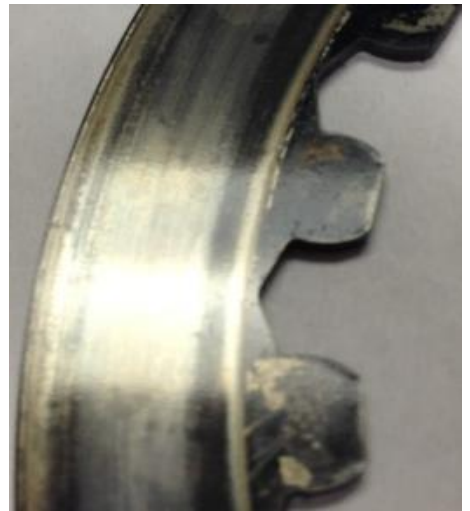
Excessive Heat (Black)
