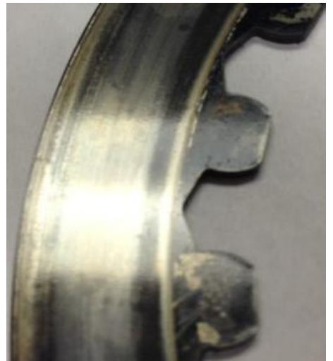
Excessive Heat (Black)
