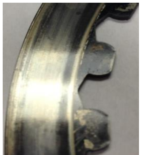
Excessive Heat (Black)
