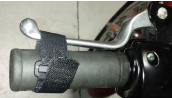
Clutch Lever Strap: to prevent unwanted launching.
