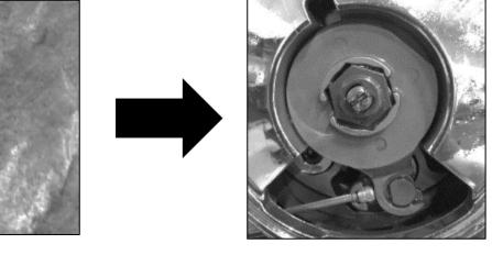
8. Reinstall the OE clutch actuating mechanism spring by pressing it onto the lock nut in the clutch actuating mechanism.
