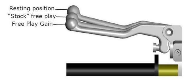
f) If you do not have the correct lever movement, see the "Adjust Free Play Gain" section.
