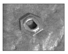
4. Turn the threaded throw-out rod clockwise until it spins freely.
