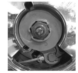
**Note:** If the lock nut will not fully index, turn the throw-out rod counterclockwise slightly until it fully indexes between the throw-out rod and the slot in the clutch actuating mechanism.
