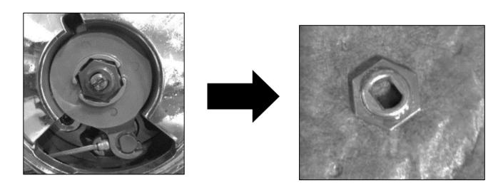
5. Turn the threaded throw-out rod **clockwise** until it spins freely.
