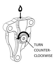
f. Compress the piston until it bottoms out. Repeat steps  $\mathbf{c}_{\cdot} - \mathbf{f}_{\cdot}$  until there is no longer air escaping from the top port when the piston is compressed.
