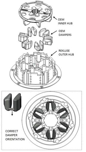
**9.** Install the new Center Hub Assembly into the motorcycle.
