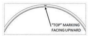
**21.** Place the OE Belleville spring onto the slider ring, with the rounded dome side facing up.
