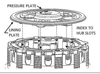
**20.** Install the OEM slider ring on the pressure plate with the "top" marking facing up. (The top side is rounded and the bottom edge is sharp.)
