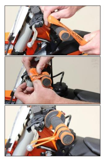
With the bike at idle in neutral, <u>quickly</u> blip (rev) the engine to at least 5,000 RPM and let it return to idle. The clutch lever should move in about 1/8" (3mm) toward the handlebar as you rev the engine. Turn the Slave Cylinder adjuster screw clockwise 1 tick at a time until optimal clutch lever movement (i.e. Free Play Gain) is achieved.
