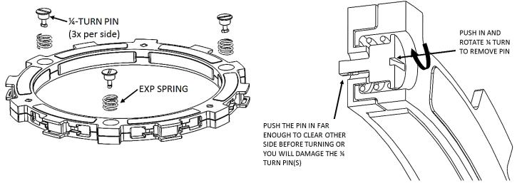
**CAUTION:** If you disassemble the EXP, bearing pads may fall out or be stuck to the ramp surfaces of the EXP bases. Take care to ensure all pads are correctly placed into wedge pockets using gentle pressure to avoid damage to the pad surfaces before reassembling the EXP. Properly seated pads will be secured in place once the EXP is reassembled. Operating the clutch without the pads in place will cause part damage or failure.
