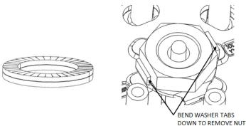
**NOTE:** Some models contain a set of lock washers instead of a tab washer. These will be removed after clutch nut and will not be reused.
