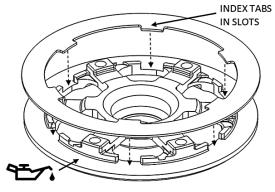
**19.** Install the pressure plate subassembly.
