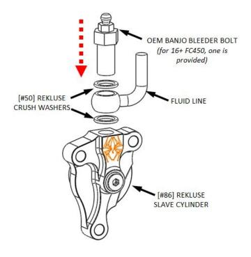
**NOTE:** Performed quickly, this method retains the fluid inside the line and makes the final bleeding step much easier.
