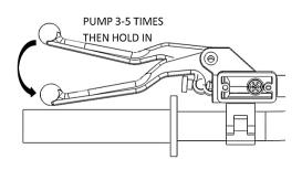
**38.** Using an 8mm wrench, open the bleed port while continuing to hold on the clutch lever at the handlebar. Air and fluid may flow from the bleed tube. Tighten the bleed port when pressure is lost.
