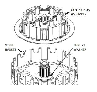
6. NOTE: The OEM dampers inside the center hub assembly shrink due to heat and use. Loose or sloppy dampers will shorten the life of your clutch. Inspect the dampers before proceeding and replace if necessary. Inspect the dampers using the procedure described in the "Read Me First" document, or by the following procedure.
