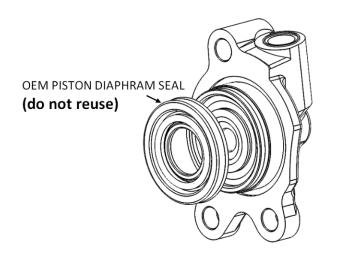
**NOTE:** The Rekluse slave cylinder comes preassembled in the kit. If the parts are separated, assemble them in the following order: Rekluse slave cylinder, supplied O-ring, then the supplied paper gasket.
