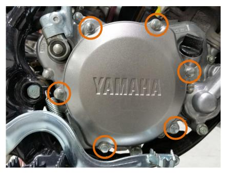
5. **CAREFULLY** remove the clutch cover to prevent damaging the clutch cover gasket or dropping the cover dowels into the engine.
