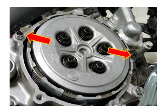
7. Remove the following OE clutch parts from the clutch basket.
