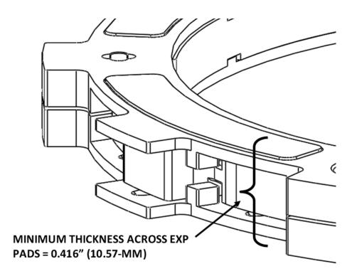
Inspect the dampers and replace them if you feel any movement between the two hubs. Refer to the section on inspecting the dampers for more information.
