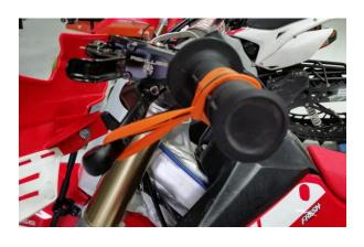
e) While still in **NEUTRAL**, quickly rev the engine between 5,000-7,000 RPM (1/2 to ¾ throttle), then let it return to idle. The end of the clutch lever **should move in about 1/8" (3mm)** toward the handlebar as you rev the engine. This is your Free Play Gain.
