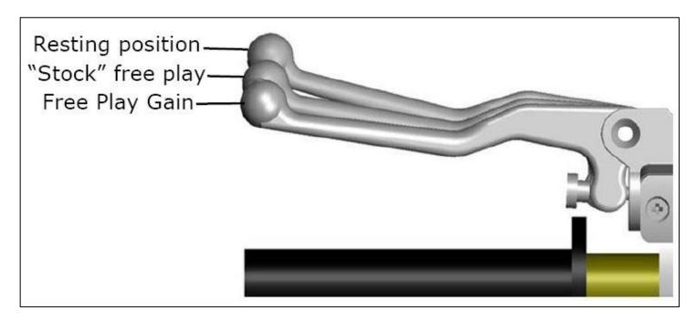
If there is too much Free Play Gain, the installed gap is too small. The bike may drag and stall because it has difficulty disengaging the clutch. It may also be difficult to shift. Too much Free Play Gain will not hurt the clutch, but it will negatively affect clutch performance.
