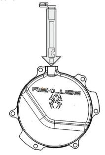
17. Transfer the pins from the OEM clutch cover into the engine case.
