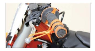
With the bike at idle in neutral, quickly blip (rev) the engine to at least half-throttle (~4,500 RPM) and let it return to idle. The end of the clutch lever should move in about 1/8" (3mm) toward the handlebar as you rev the engine.
