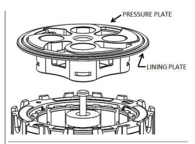
15. Install the pressure plate springs, torqueing the screws to 9 ft-lb (12 N-m).
