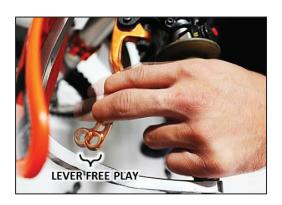
"Free Play Gain" is the increase of lever free play as the auto-clutch engages. This happens when the RPM increase from idle through around half-throttle (4,500 RPM). Free Play Gain is caused by the expansion of the EXP disk which lifts the pressure plate away from the throw-out assembly.
