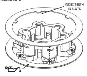
14. Install the pressure plate and lining plate assembly.
