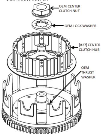
**NOTE**: If the OEM thrust washer is not in place, it is probably stuck to the backside of your OEM center clutch hub.
