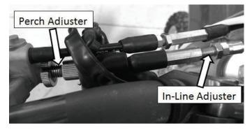
21. In the next section, you will make adjustments using the front jam nut and perch adjuster to set the desired Installed-Gap based on the lever Free Play Gain. Once this is established and everything functions well, you will tighten the adjuster jam nuts to secure your cable
