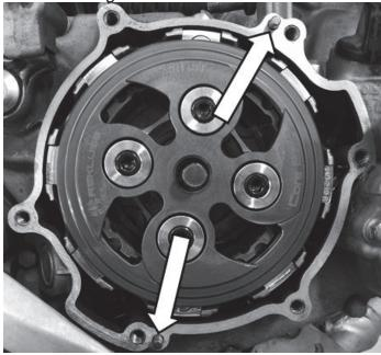
18. Install the Rekluse clutch cover, reusing the OEM gasket, and torque bolts to OEM specifications.
