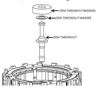
**NOTE:** The hole in the throw-out bearing is bigger than the throw-out so it "floats" on the throw-out. The bearing will seat in when it has pressure from the pressure plate.
