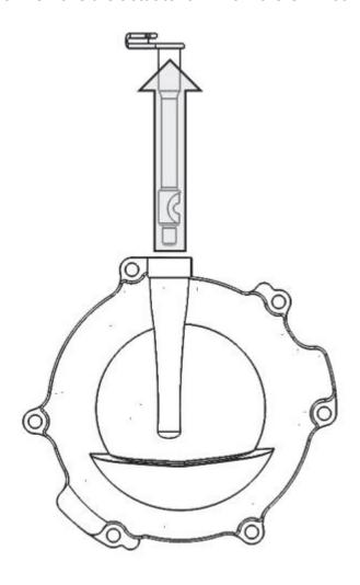
7. Remove the OEM clutch parts named in the following diagram. Leave the basket installed.
