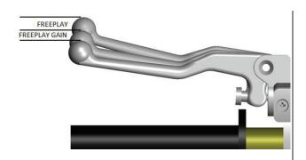
Optimal Freeplay Gain yields ~1/8" (3mm) of clutch lever movement, measured at the ball end of the lever. This measurement at the lever correlates to achieving the ideal installed gap, so you will use the Freeplay Gain measurement to accurately set the installed gap.
