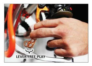
"Freeplay Gain" is the increase of lever freeplay as the auto-clutch engages. This happens when the RPM increase from idle through around 5.000 RPM with either configuration. Freeplay Gain is caused by the expansion of the EXP disk which lifts the pressure plate away from the throwout assembly.
