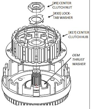
**NOTE**: If the OE thrust washer is not in place, it is probably stuck to the backside of your OE center clutch hub.
