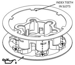
**11.** Install this pressure plate subassembly.
