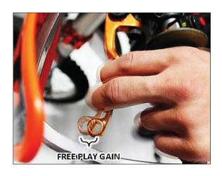
The following steps explain two ways to check Freeplay Gain. One will use the rubber band that has been included in the clutch kit and the other explains using your hand, which you will perform before every ride.
