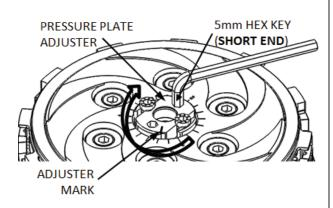
**NOTE:** As you turn the adjuster, the clutch may slip and start to spin before you reach 1-full turn. Placing the bike in gear and holding the rear brake or tire will provide leverage to prevent clutch spin while adjusting.
