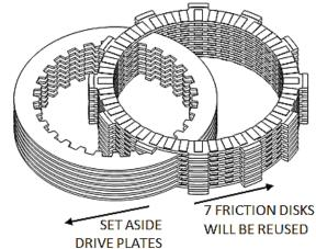
Inspect the friction disks for signs of heat or wear. Replace if they are burnt or worn. For most models, new friction disks can be purchased from Rekluse.
