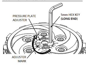
**14.** At this point, make a note of where the tick mark on the Adjuster aligns with the tick marks on the Pressure Plate. This is what's called the **STARTING POINT.**
