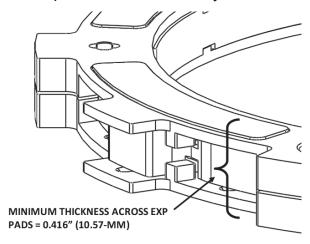
Repeat the break-in procedure anytime the friction disks or EXP bases or wedges are replaced. Always soak friction disks or EXP bases in oil for at least 5 minutes before installing.
