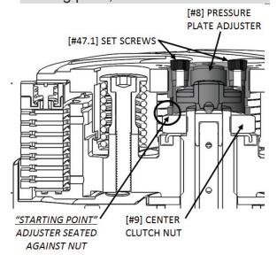
16. Now, insert the short end of the 5-mm hex key into the pressure plate adjuster, and turn it clockwise one full turn plus 2 tick marks past the starting point (aka "1+2").
