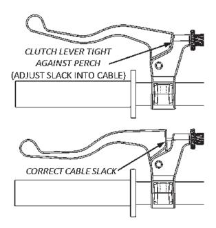
If there is not enough adjustment at the lever perch, you may need to make further adjustment using the in-line cable adjuster.
