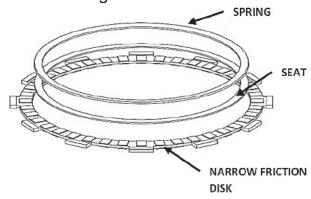
STOCK Clutch Pack Cutaway View
