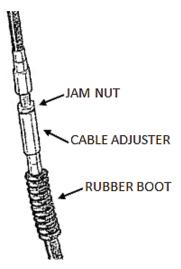
NOTE: The Pressure Plate Adjuster should bottom out and lift against the center clutch nut, not the throwout. Slack in the clutch cable ensures that you'll find the correct starting point, not a false one.
