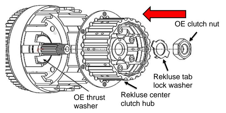
3. Install the new Rekluse tab washer with the bent tabs facing down, aligning with the holes in the hub. Only use the supplied lock tab washer under the OE center clutch nut when installing the hub.
