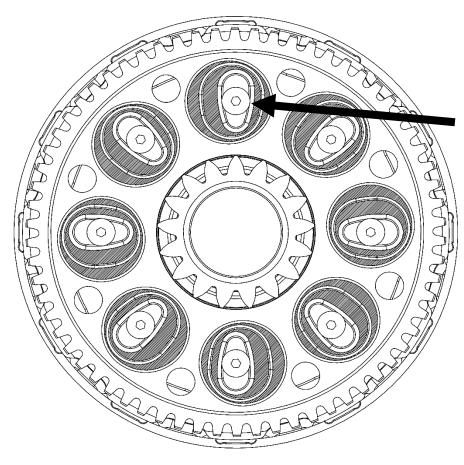
Starting from the top install dampers with the thick side of the damper to left of the standoff and logo facing up 2. Reinstall the OE ring gear. The ring gear may fit snugly and will likely require using a soft mallet to tap it on until it seats all the way against the basket.
