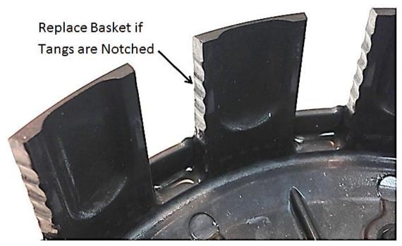
Do not use baskets that have been filed, machined, or modified on the tangs.
