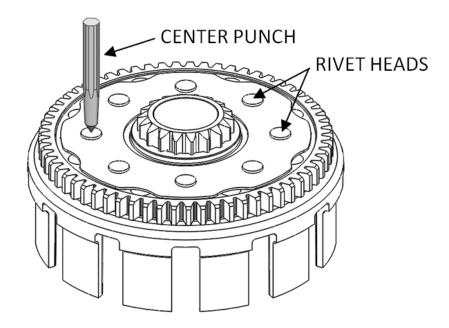
2.Use the supplied drill bit to drill out the heads of all the rivets. Set your drill to 300-400 RPM and use proper cutting fluid or oil for best results.
