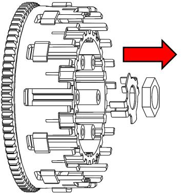
14. Remove the center hub and the clutch basket. Separate the thrust washer as it will be reused later.
