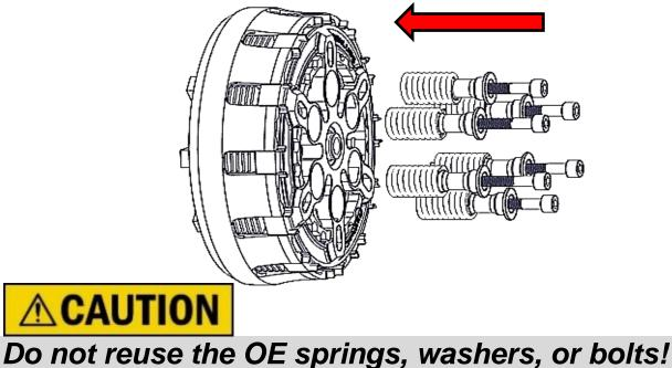
7.Use a torque wrench and socket to torque the cap screws by lightly tightening the screws in small increments. Torque the cap screws to **9 ft-lb (12 N-m)**.
