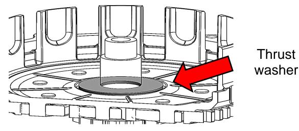
2. Install the new Rekluse center hub into the clutch basket.
