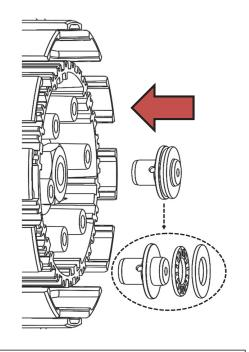
If the washer is missing: Check to see if it is stuck to the backside of the OE pressure plate
