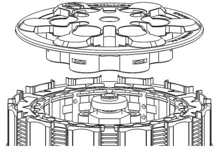
5. Install the pressure plate springs, followed by the screw sleeves and socket head cap screws (5 or 6 depending on the bike). See setup sheet for spring options included in kit. If using two different spring colors (6 spring clutches only), be sure to alternate the springs by color in every other pocket.
