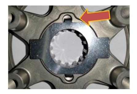
4. Install the OE center clutch nut.
