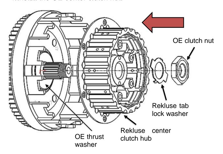
5. Using the socket and torque wrench, torque the center clutch nut to **50 ft-lb (68 N-m)**.
