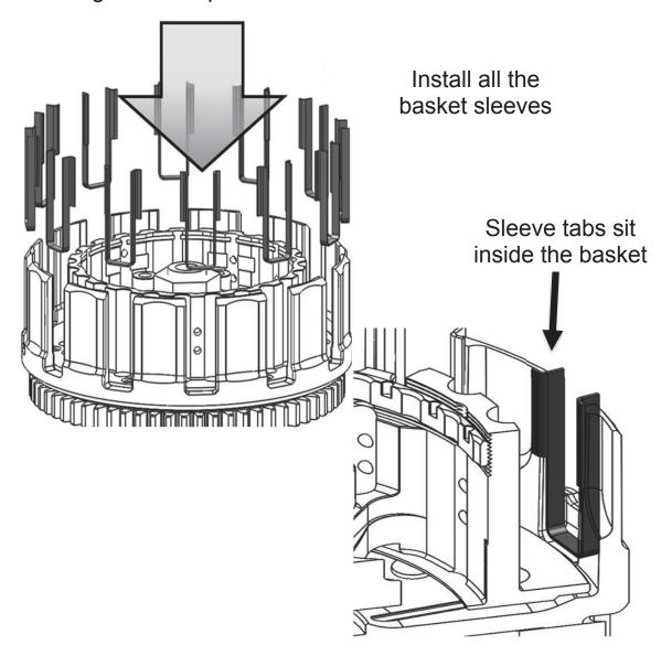
**Note:** If the basket sleeves fall forward while installing the clutch pack, us a pick to push them back into place. When seated in the basket, the sleeves may stick above or below flush with the top of the basket depending on the bike model. This is normal.
