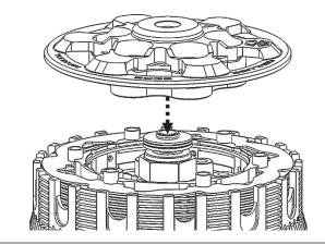
**12.** Install the Rekluse pressure plate springs and torque the pressure plate bolts.
