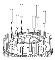
**8.** Install the first TEC drive plate in the orientation shown (all drive plates will follow this orientation).
