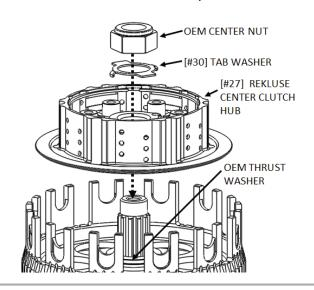
**6.** Torque the nut to OEM specification, and bend up **both** tabs of the tab washer using channel-lock pliers.
