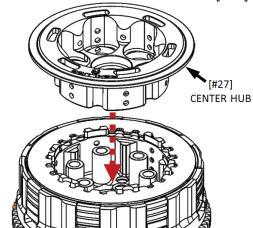
To get the spline in the hub to line up with the mainshaft spline, gently rotate the hub back and forth while installing it until the splines mesh and the hub drops into place. DO NOT force the hub into place or damage will occur.
