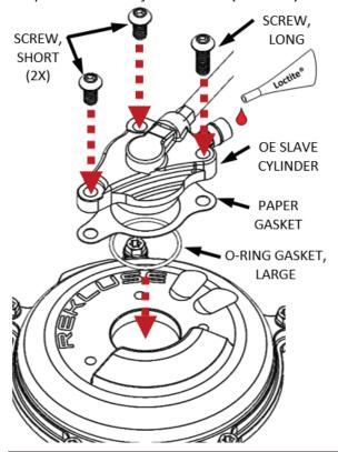
**NOTE:** The longer screw *MUST* be placed in the hole location where the slave cylinder housing is thickest (rightmost side of the slave cylinder).
