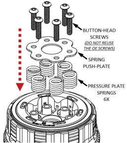
DO NOT reuse the OE screws, as interference with the clutch cover will occur.
