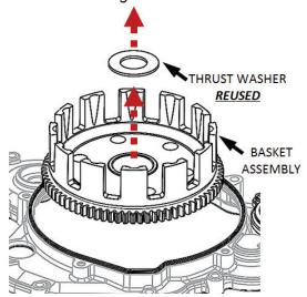
**NOTE:** If the thrust washer is not in the basket, it is likely stuck to the backside of the hub that was removed in the previous step.
