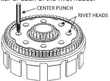
**10.** Using the drill bit provided, drill the heads off of each rivet, so that the backing plate can be removed from the assembly.
