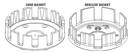
The Rekluse Core components, including the Basket [#24], Center Hub [#27], and Pressure Plate [#5], are compatible with both the CoreManual and CoreEXP (auto) clutches. CoreManual can be converted to a CoreEXP auto-clutch by purchasing the EXP disk and the Adjustable Slave Cylinder assemblies from Rekluse. Follow the directions in the CoreEXP Installation Guide to properly install and check for function.
