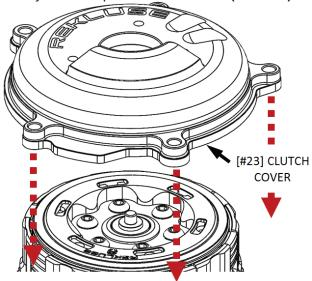
**NOTE:** The *OE* clutch cover is *not* compatible with any Rekluse clutch product (CoreEXP or CoreManual) because it does not provide adequate clearance to the moving parts. The Rekluse clutch cover *must* be used with any Rekluse clutch product.
