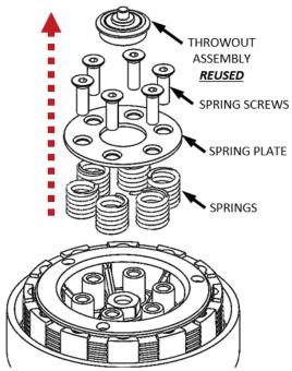
**7.** Using a 17mm socket, remove the center hub bolt. Then, lift the core of the clutch out by gripping the spring posts and pulling upward.
