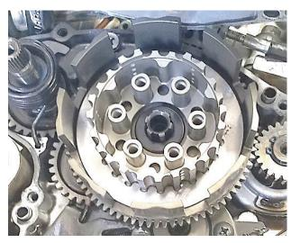
27. Install the Rekluse clutch pack as shown, starting and ending with a steel drive plate [#67]. 7x total drive plates will be used, 5x stock and 2x provided.
