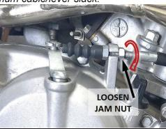
**NOTE:** The clutch cable does not have to be removed from the clutch cover to enable access to the clutch. See the next steps for the procedure to tilt the cover out of the way.
