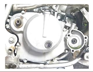
**34.** Replace the water pump impeller. Torque to **8.3 N-m (6 ft-lb)**.
