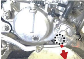
4. Making sure that the engine/coolant is not hot, twist open the radiator cap to help evacuate all the coolant from the system into the container.
