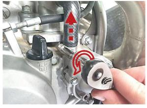
**11.** Both the water pump housing and the coolantout hose can be moved out of the way of the clutch cover by gently tucking them between the engine and the exhaust pipe.
