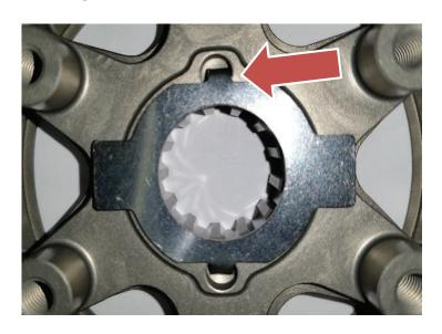
4. Install the OE center clutch nut.
