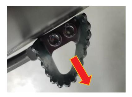
5. Using an 8 mm socket, remove the OE clutch cover. Pay close attention to the length and location of the OE screws so they can each be returned to the same location.
