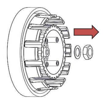
12. Remove the center hub from the clutch basket while leaving the thrust washer on the main shaft.
