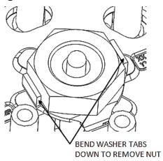
10. Remove the center clutch nut with an impact wrench or breaker bar, and a socket. Set aside. The OE clutch nut will be reused.
