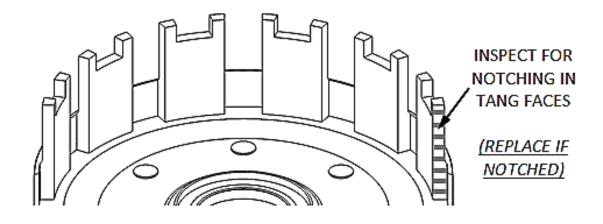
**Note:** Through extensive testing, Rekluse recommends replacing the OE clutch basket--even if the basket is in good condition. Billet Clutch Baskets are available from Rekluse and are specifically designed to ensure the longevity of your clutch.
