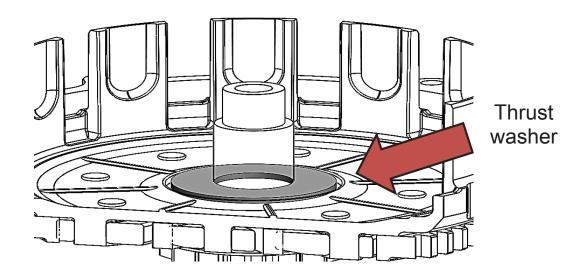
13. Inspect the clutch basket for spring damper play or notching. Do not install sleeves or use product with a notched basket. Notched basket tang faces or worn dampers can cause the sleeves to break. Do not use baskets that have been filed, machined, or modified on the tangs. Replace basket if necessary.
