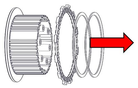
Separate the OE clutch pack. All the friction disks will be reused. All the drive plates will be replaced with Rekluse steel drive plates.
