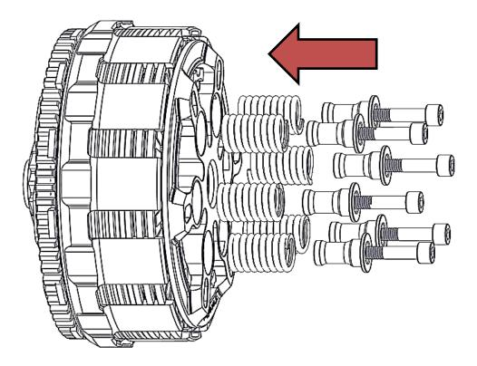
5.Use a torque wrench and socket to torque the cap screws by lightly tightening the screws in small increments. Torque the cap screws to 9 ft-lb (12 N-m).
