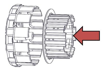
3. Install the new Rekluse tab washer with the bent tabs facing down, aligning with the holes in the hub. *Only use the supplied lock tab washer under the OE center clutch nut when installing the hub.*
