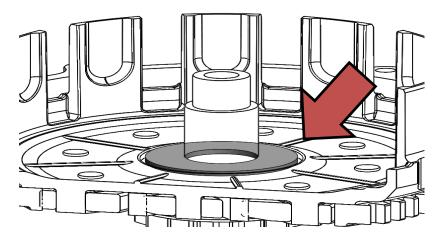
2. Install the new Rekluse center hub into the clutch basket.
