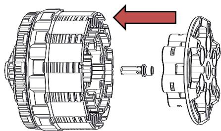
4. Install the pressure plate springs, followed by the screw sleeves and socket head cap screws. Alternative spring options are available from Rekluse if desired. The springs provided are the recommended setting for optimum balance of performance and lever feel.
