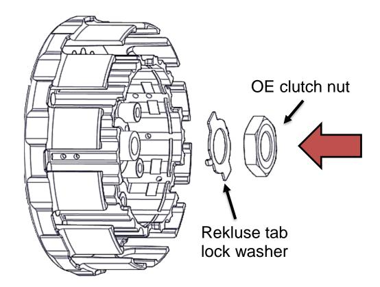
5. Using the socket and torque wrench, torque the center clutch nut to **50** ft-lb (**68** N-m).
