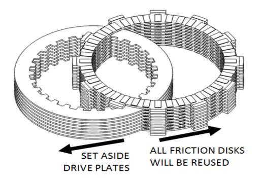
7. Inspect the friction disks for signs of heat or wear. Replace if they are burnt or worn.
