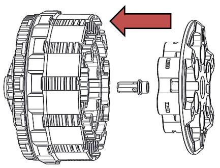
4. Install the pressure plate springs, followed by the screw sleeves and socket head cap screws (5 or 6 depending on the bike). Alternative spring options are available from Rekluse if desired. The springs provided are the recommended setting for optimum balance of performance and lever feel.
