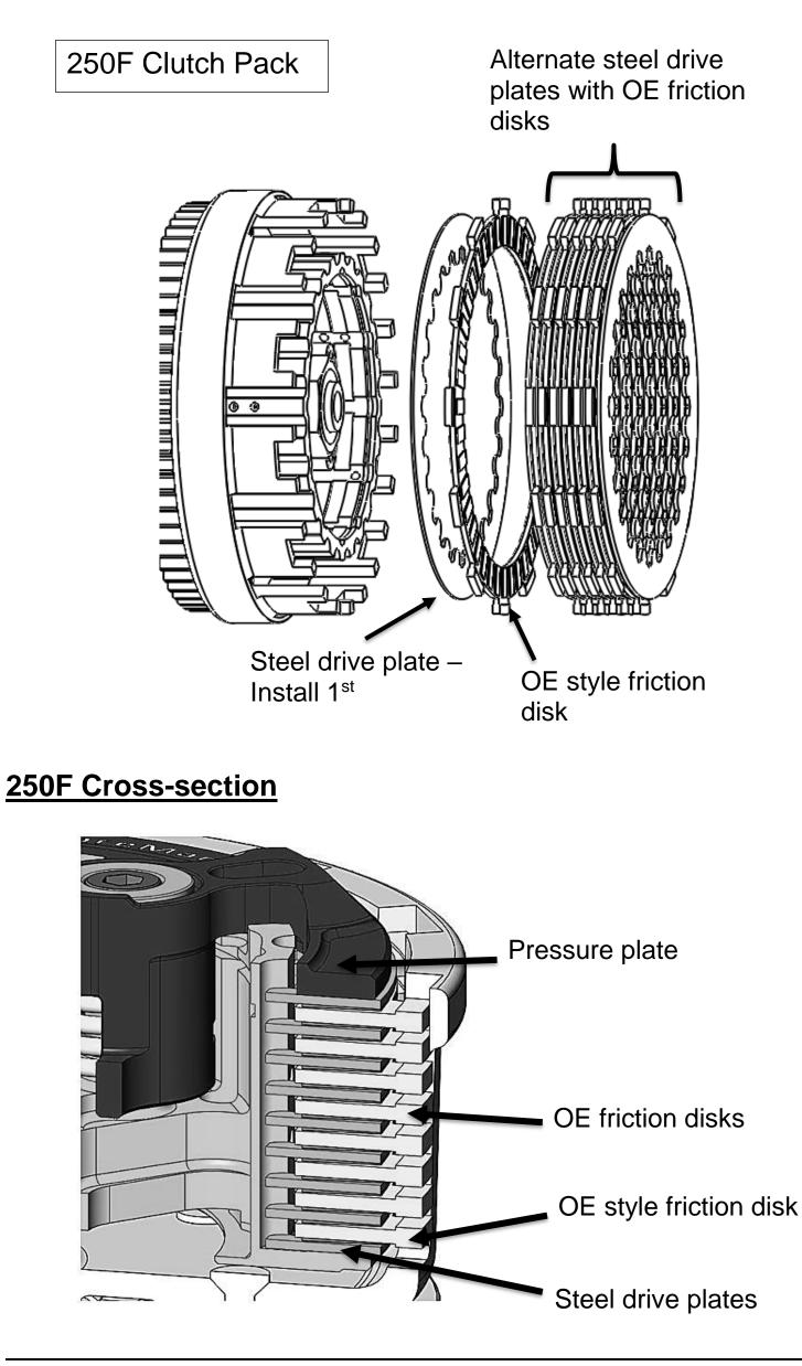
3. Reinstall the OE throw-out, then install the Rekluse pressure plate.
