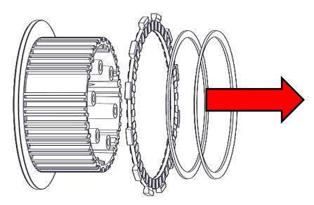
6. Separate the OE clutch pack. All the friction disks will be reused. All the drive plates will be replaced with Rekluse steel drive plates.
