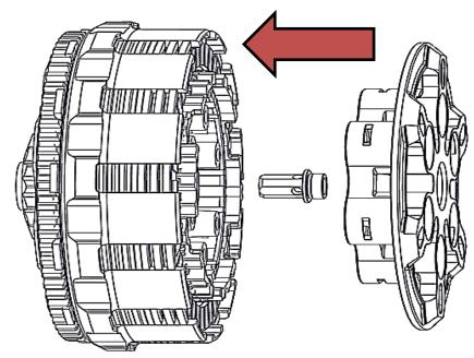
4. Install the pressure plate springs, followed by the screw sleeves and socket head cap screws (5 or 6 depending on the bike). Alternative spring options are available from Rekluse if desired. The springs provided are the recommended setting for optimum balance of performance and lever feel.
