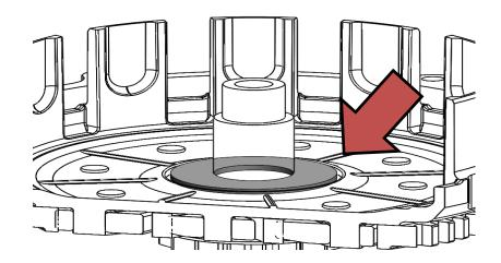
2. Install the new Rekluse center hub into the clutch basket.
