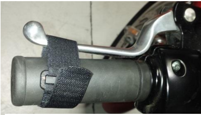
Clutch Lever Strap: to prevent unwanted launching.
