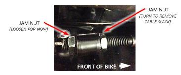
**21.** Once all the cable slack is gone, tighten the front jam nut about 3 more turns, so that the clutch actuator arm starts to move. This is a decent starting point for finding the correct installed gap.
