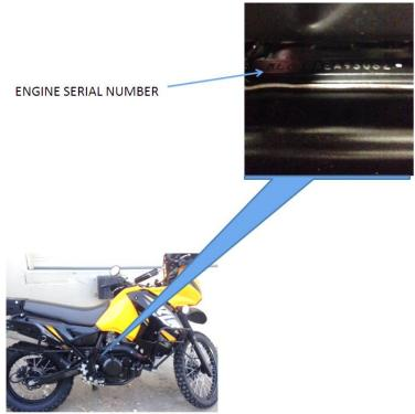
Engine serial number is located just above the clutch cover and underneath the exhaust on the top surface of the engine.
