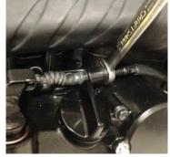
Using needle-nose pliers, grip and feed the 8. clutch cable through the actuator arm to disconnect the clutch cable from the actuator.
