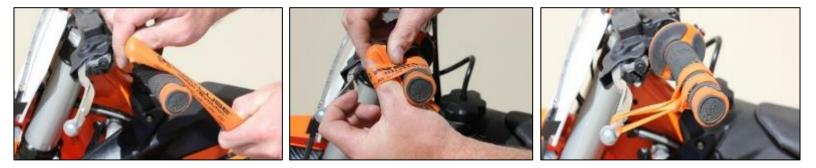
e) While still in **NEUTRAL**, quickly rev the engine to about 5,000 RPM, then let it return to idle. Notice the movement in the clutch lever when the engine is revved. This is your Free Play Gain.
