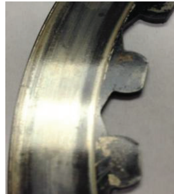
Excessive Heat (Black)
