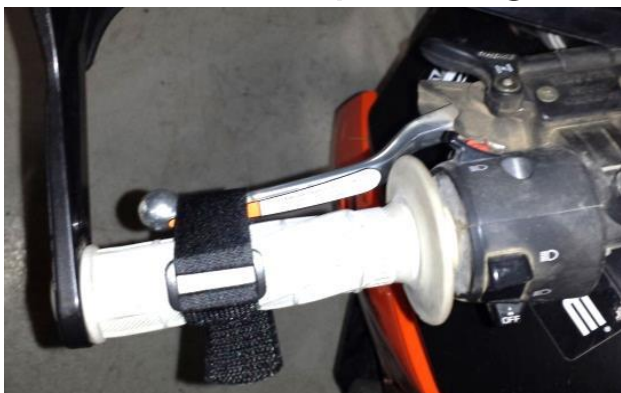
Clutch Lever Strap: to prevent unwanted launching.
