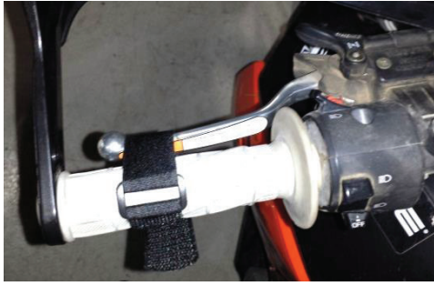
Clutch Lever Strap: to prevent unwanted launching.
