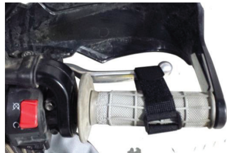
Brake Lever Strap: for use as a parking brake.
