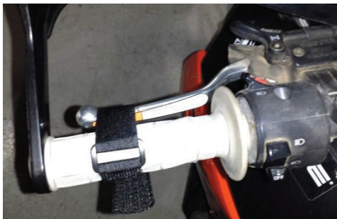
Clutch Lever Strap: to prevent unwanted launching.
