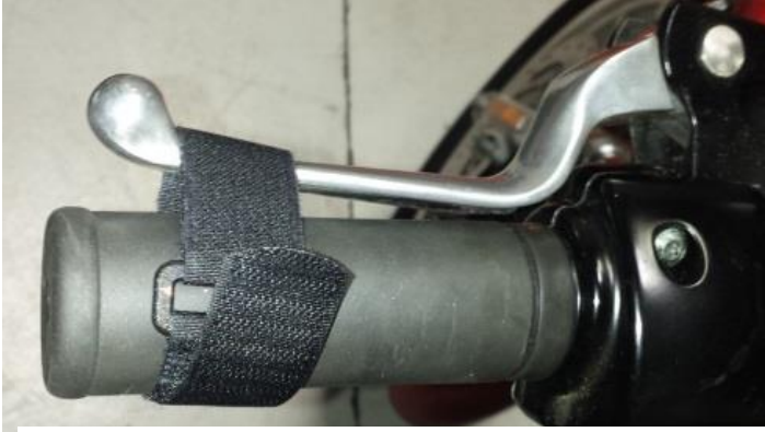
Clutch Lever Strap: to prevent unwanted launching.
