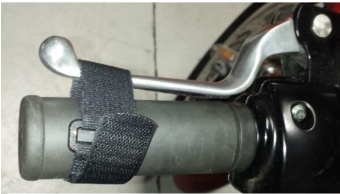
Clutch Lever Strap: to prevent unwanted launching.
