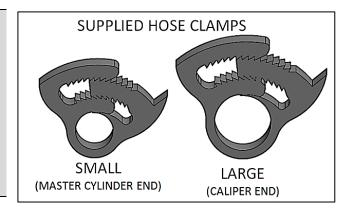
4. Place an 8mm box end wrench over the bleed nipple and slide the large tubing clamp over the hose on one of the syringes (but don't clamp it yet), then slip the syringe hose over the caliper bleed nipple.
