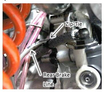
**NOTE**: The brake line comes preassembled with a length of thermal shielding on the banjo end. Make sure that this shielding is slid down the line toward the banjo before securing the line with zip ties. The shield is intended to protect the brake line from the heat of the exhaust pipe.
