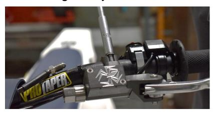
**NOTE:** It can be helpful to remove the clutch master cylinder from the bar after installing the line to assist in the bleeding of the Rekluse master cylinder
