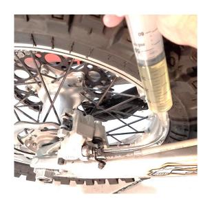
**9.**Keep pushing fluid through the system while it starts to fill the syringe up at the master cylinder. Push until no more air bubbles are coming out of the master cylinder bleed port, then close the bleed nipple at the caliper.
