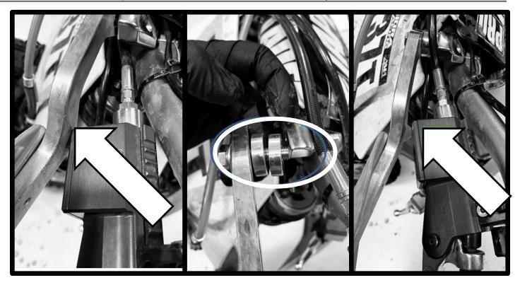
**2.** After determining the desired lever positions, including the clutch lever perch, re-tighten the handlebar clamps evenly. Tighten the clamp screws to **7 ft-lbs (10N-m).**
