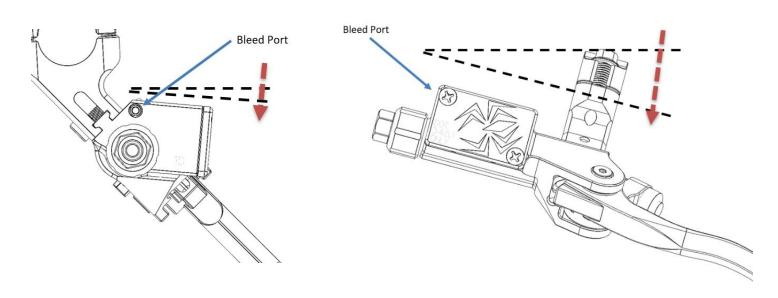
**NOTE**: This can also be achieved by removing the housing from the bars and being allowed to hang in a proper orientation
