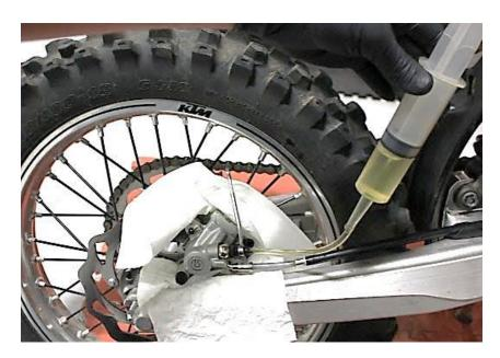
2. At the Rekluse master cylinder, remove the top bleed port screw using a 2.5mm Allen
