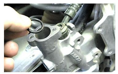
**NOTE:** Ensure the O-ring seats properly in the reservoir. It can get caught on the sight glass cutout and tear. This will prevent the system from holding brake pressure.
