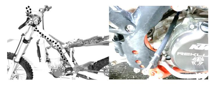
**4.**From the Brake Line Kit, install the fittings at the rear master cylinder as shown. The banjo fitting on the line should be sandwiched between two square-ring seals on the banjo bolt.
