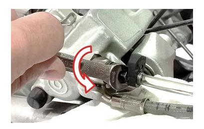
**8.** Slowly start to push fluid through the system with the syringe at the caliper.
