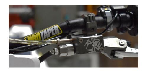
**NOTE**: If the fitting leaks after being tightened hand tight, then pliers can be used to tighten the fitting into the housing. Be careful not to over-tighten and snap the fitting off in the housing.
