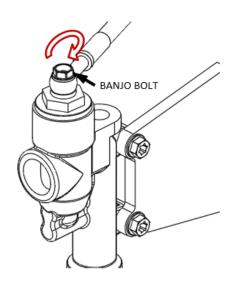
**6.**Using an 8mm socket, mount the Rekluse master cylinder onto the left handlebar. This does not have to be its permanent location but is a good location for routing the brake line and bleeding the system.
