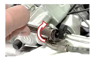
**NOTE**: It can be helpful to tap the brake line and master cylinder, pump the lever rapidly, and rotate the master cylinder to help dislodge any remaining air bubbles.
