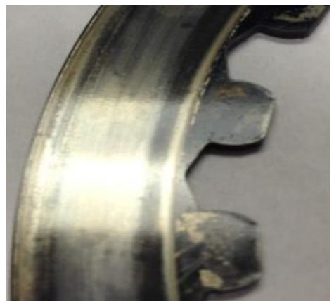
Excessive Heat (Black)
