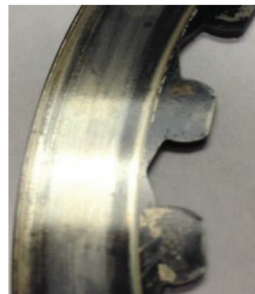
Excessive Heat (Black)
