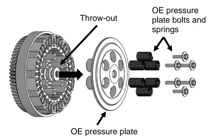
**Note:** Throw-out washers can stick to the back of the pressure plate. Be sure to reinstall any throw-out washers back onto the throw-out.
