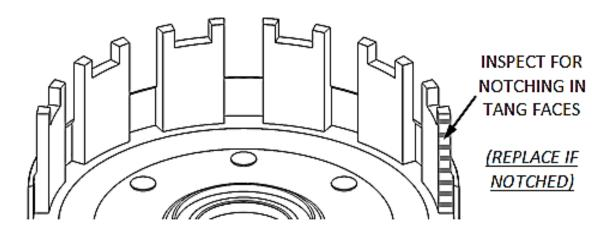
**Note:** If the basket is notched or worn, Rekluse recommends replacing it with a Rekluse Billet Clutch Basket (available for most models).
