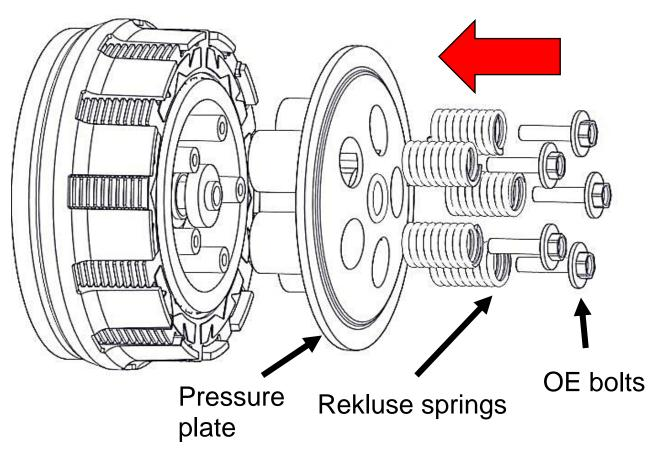
**Note:** For Yamaha YZ250F (2019+), YZ250FX (2020+), & WR250F (2020+) when installing the pressure plate align the indent in the pressure plate with the indent in the center hub.
