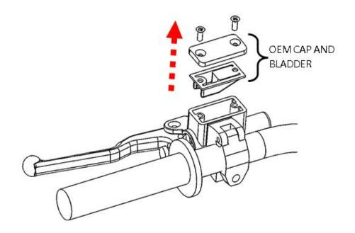
3. Top off the master cylinder with the recommended clutch fluid.
