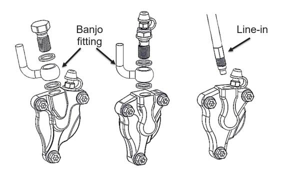
3. Attach the clutch fluid line to the Rekluse slave cylinder using the OE banjo bolt and the 2 new Rekluse crush washers (if applicable). Make sure the banjo fitting is sandwiched between the 2 crush washers.
