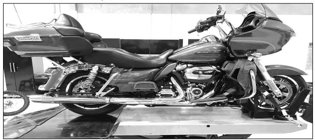
2.Loosen the exhaust system (muffler and header assembly) to gain access to the transmission side cover. Removing the exhaust heat shields will also give more clearance and help prevent damage from brake fluid.
