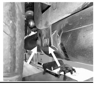
ii. Apply Loctite to the hinged clamp bolt and torque to 25 ft lbs
