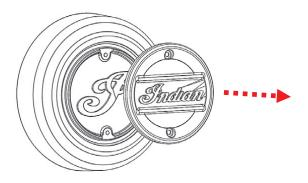
2. Install the Rekluse derby cover onto the clutch cover using the OE cover screws.
