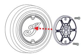
3. Apply Loctite 243 or equivalent to the screws. Lightly tighten bolts in small increments, then torque to **9 ft-lb (12 N-m)**.
