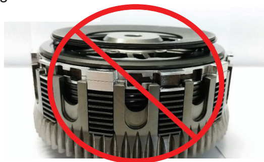
Incorrect – The Belleville spring is upside down.
