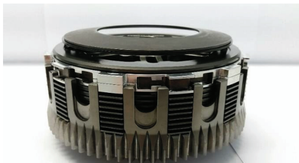
Correct – The Belleville spring sits flat against the slider ring.
